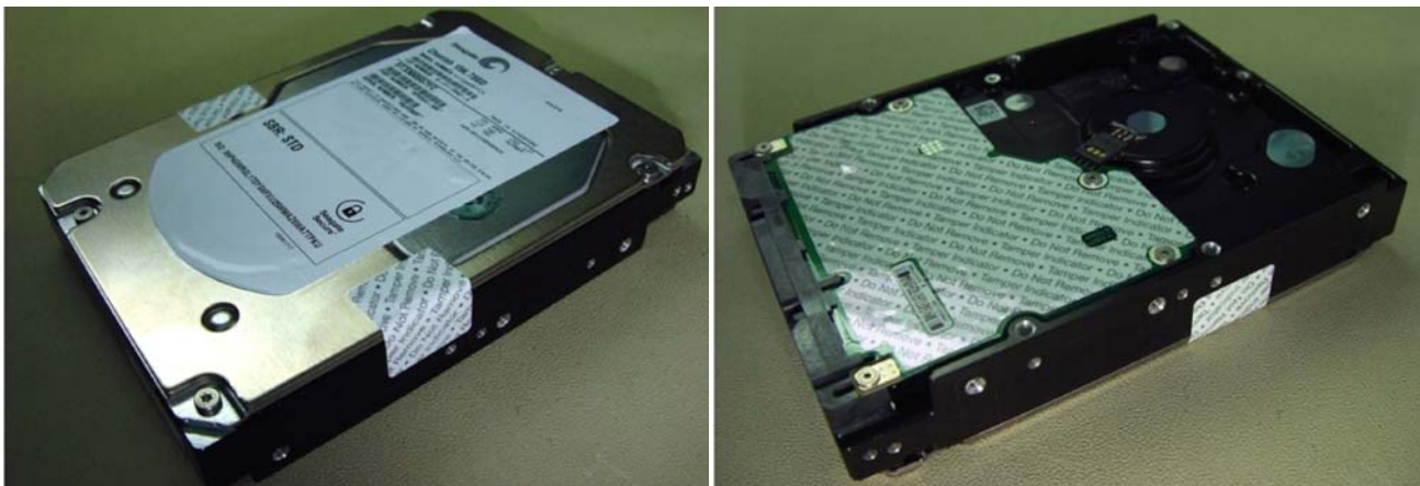
Figure 16. Example of FIPS tamper evidence labels.
