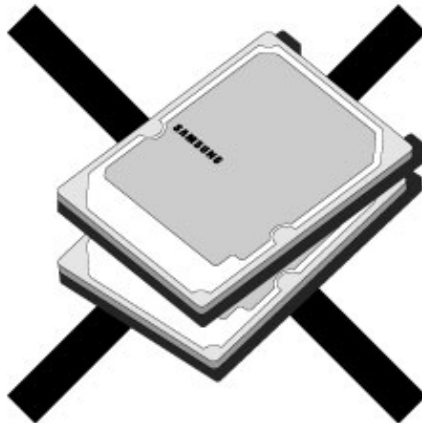
Fig. 9-3: HDD handling guide -Do Not Stack!
