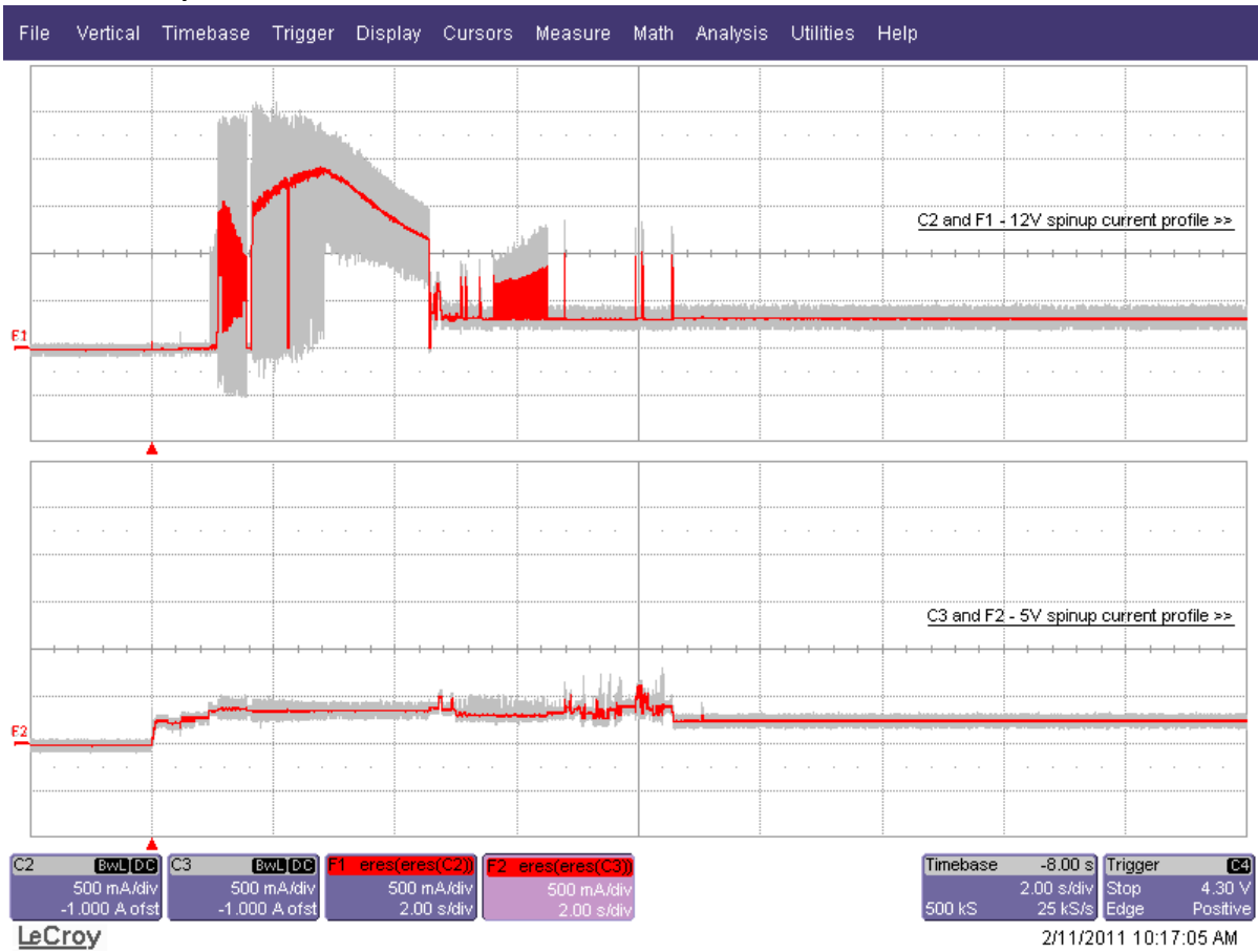
Figure 2. Typical 1TB model 5V & 12V startup and operation current profiles
